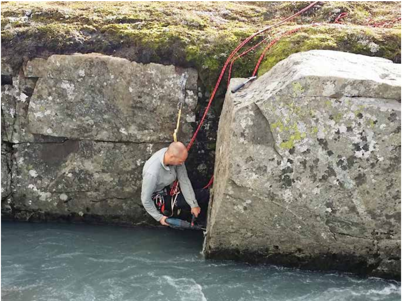
John Hulth from the University of Oslo rigging a stilling well for a pressure logger in a stream near Finse. The data will be used to determine streamflow in one of the rivers coming from the glacier Hardangerjøkulen, as part of the EVOGLAC project.
