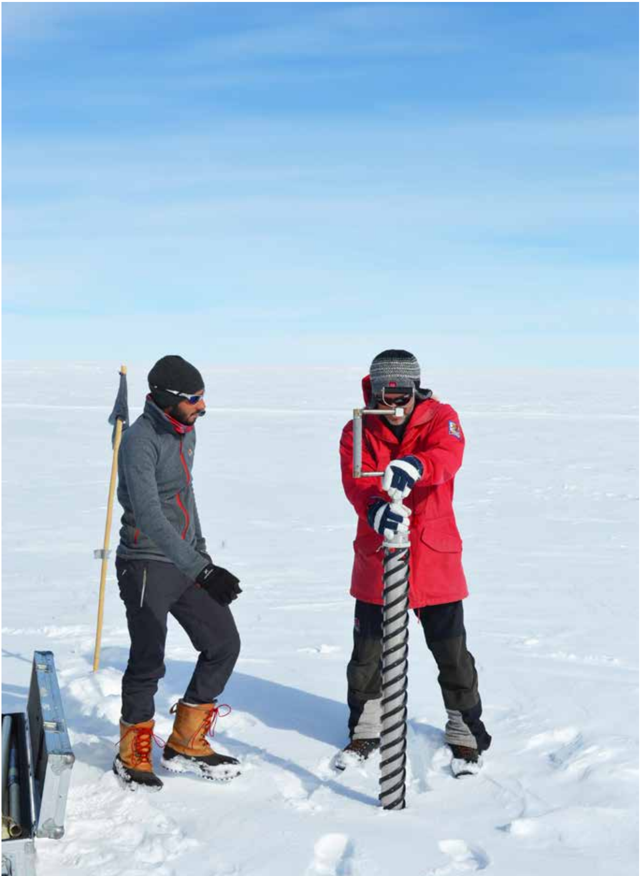
❶ Drilling in north-east Greenland. Kerim Nisancioglu, UiB and the Bjerknes Centre, and Niccolo Maffezzoli, University of Copenhagen. The first metres of ice were drilled by hand from the surface. The next 70 metres or so were drilled by a mechanical drill giving individual cores of a little more than one metre each.
